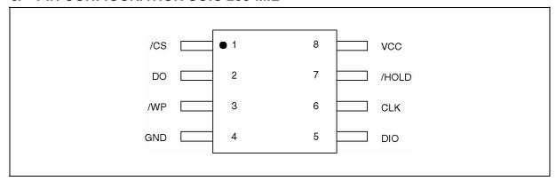
Figure 1a. W25X16 and W25X32 Pin Assignments, 8-pin SOIC (Package Code SS)
