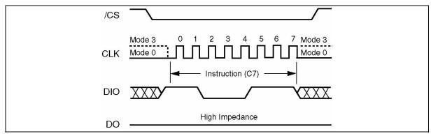
Figure 14. Chip Erase Instruction Sequence Diagram
