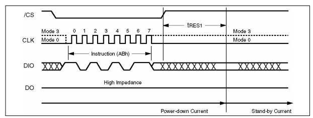
Figure 16. Release Power-down Instruction Sequence
