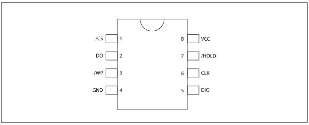
Figure 1c. W25X16, W25X32, W25X64 Pin Assignments, 8-pin PDIP (Package Code DA)
