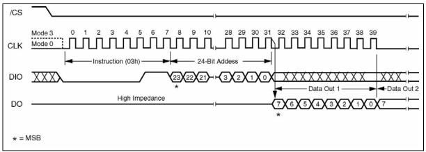
Figure 8. Read Data Instruction Sequence Diagram
