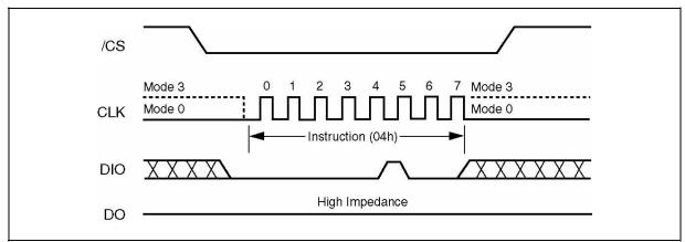
Figure 5. Write Disable Instruction Sequence Diagram
