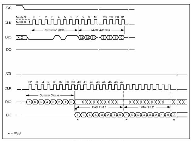
Figure 9. Fast Read Instruction Sequence Diagram
