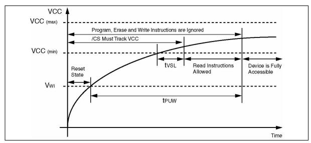
Figure 20. Power-up Timing and Voltage Levels
