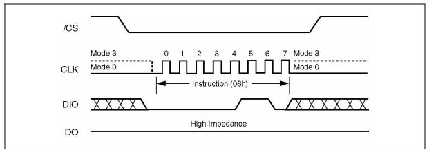
Figure 4. Write Enable Instruction Sequence Diagram
