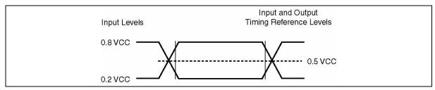
Figure 21. AC Measurement I/O Waveform
