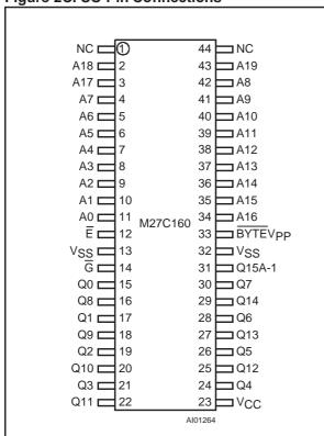
Figure 2B. PLCC Pin Connections
