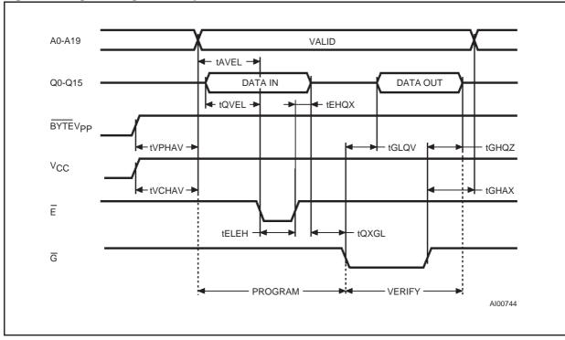
Figure 8. Programming and Verify Modes AC Waveforms
