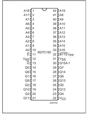
Figure 2C. SO Pin Connections
