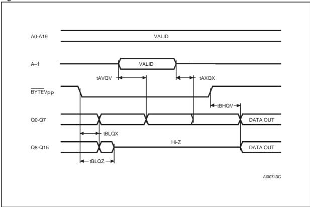
Note: Chip Enable  $(\overline{E})$  and Output Enable  $(\overline{G}) = V_{IL}$ .
