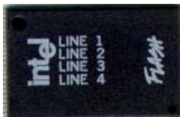
Figure 7. New Mark for Pin-1 Indicator: 40-Lead 8/16 Mb TSOP and 48-Lead 8/16/32 Mb TSOP
