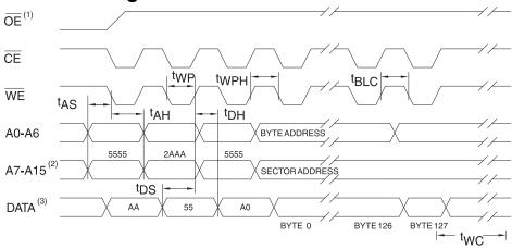
Notes: 1.  $\overline{OE}$  must be high when  $\overline{WE}$  and  $\overline{CE}$  are both low.
