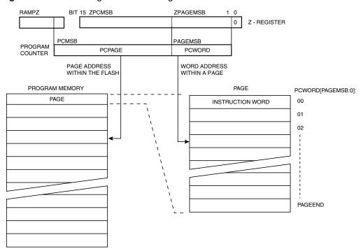
Figure 133. Addressing the Flash During SPM<sup>(1)</sup>
