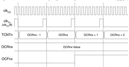
Figure 55. Timer/Counter Timing Diagram, Setting of OCFnx, with Prescaler ( $f_{clk_1/O}/8$ )
