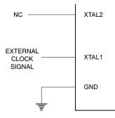
When this clock source is selected, start-up times are determined by the SUT fuses as shown in Table 16.
