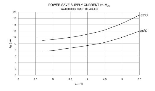
Figure 174. Power-save Supply Current vs.  $V_{\text{CC}},$  Watchdog Timer Disabled
