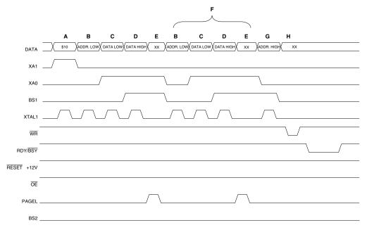
Figure 136. Programming the Flash Waveforms
