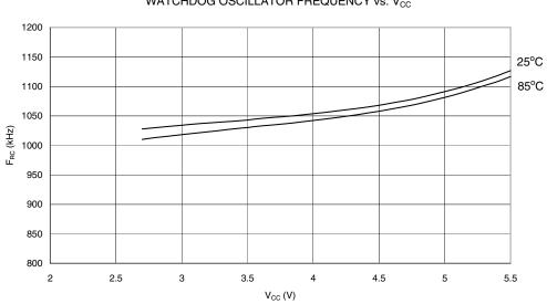
WATCHDOG OSCILLATOR FREQUENCY vs.  $V_{\text{CC}}$
