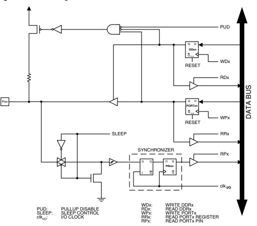
Note: 1. WPx, WDx, RRx, RPx, and RDx are common to all pins within the same port. clk<sub>I/O</sub>, SLEEP, and PUD are common to all ports.
