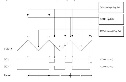
Figure 39. Phase Correct PWM Mode, Timing Diagram
