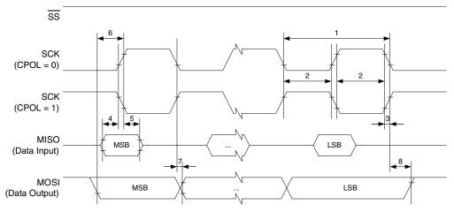
Figure 155. SPI Interface Timing Requirements (Slave Mode)
