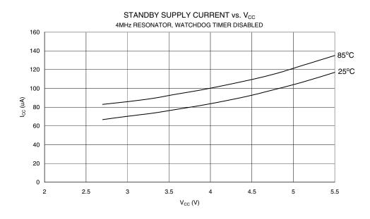
Figure 178. Standby Supply Current vs.  $V_{\text{CC}},\,4$  MHz Resonator, Watchdog Timer Disabled
