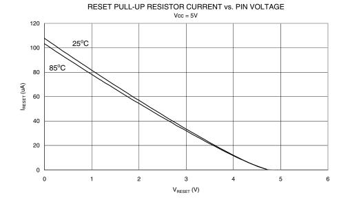
Figure 182. Reset Pin Pullup Resistor Current vs. Input Voltage,  $V_{CC} = 5V$
