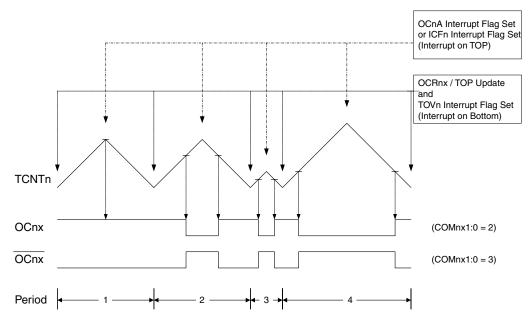
Figure 53. Phase and Frequency Correct PWM Mode, Timing Diagram
