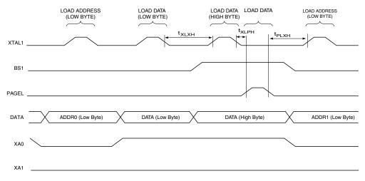
Note: The timing requirements shown in Figure 140 (i.e. t<sub>DVXH</sub>, t<sub>XHXL</sub>, and t<sub>XLDX</sub>) also apply to loading operation.
