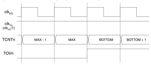
Figure 68 shows the same timing data, but with the prescaler enabled.
