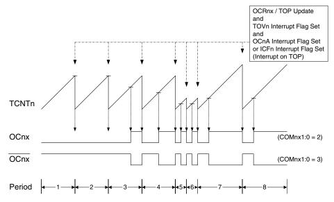
The Timer/Counter Overflow Flag (TOVn) is set each time the counter reaches TOP. In addition the OCnA or ICFn flag is set at the same timer clock cycle as TOVn is set when either OCRnA or ICRn is used for defining the TOP value. If one of the interrupts are enabled, the interrupt handler routine can be used for updating the TOP and compare values.
