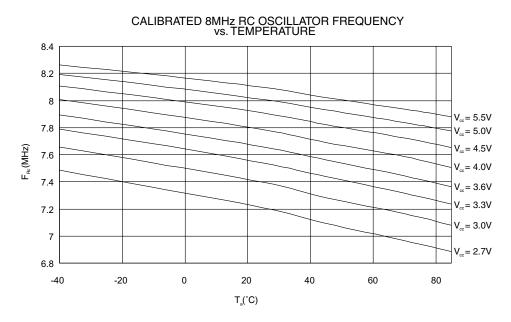
**Figure 202.** RC Oscillator Frequency vs. Operating Voltage (the devices are calibrated to 8 MHz at Vcc = 5V, T=25c)
