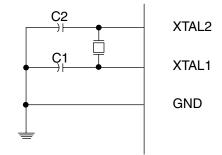
The Oscillator can operate in three different modes, each optimized for a specific frequency range. The operating mode is selected by the fuses CKSEL3..1 as shown in Table 8.
