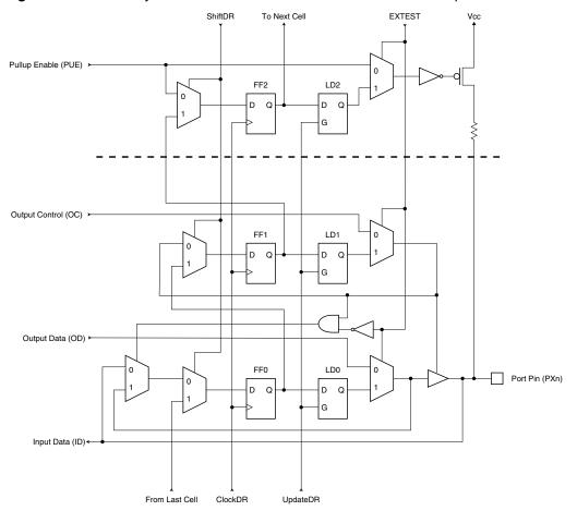
Figure 123. Boundary-scan Cell for Bi-directional Port Pin with Pull-Up Function.
