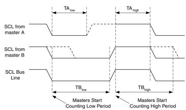
Figure 91. SCL Synchronization between Multiple Masters
