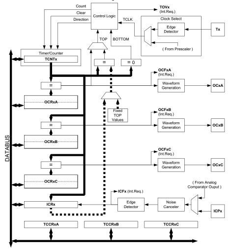
Figure 45. 16-bit Timer/Counter Block Diagram
