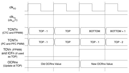
Figure 57 shows the same timing data, but with the prescaler enabled.
