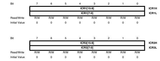
The Input Capture is updated with the counter (TCNTn) value each time an event occurs on the ICPn pin (or optionally on the Analog Comparator Output for Timer/Counter1). The input capture can be used for defining the counter TOP value.
