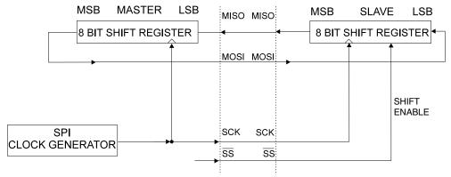
Figure 75. SPI Master-Slave Interconnection
