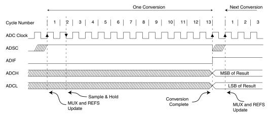
Figure 111. ADC Timing Diagram, Free Running Conversion
