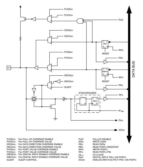
Note: 1. WPx, WDx, RLx, RPx, and RDx are common to all pins within the same port. clk<sub>I/O</sub>, SLEEP, and PUD are common to all ports. All other signals are unique for each pin.
