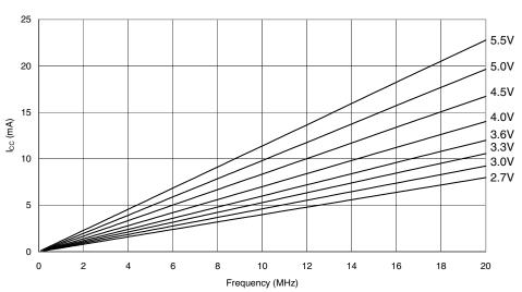
IDLE SUPPLY CURRENT vs. FREQUENCY
