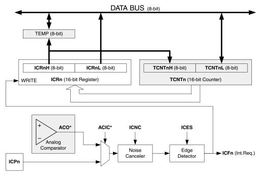
Note: The Analog Comparator Output (ACO) can only trigger the Timer/Counter1 ICP – not Timer/Counter3.
