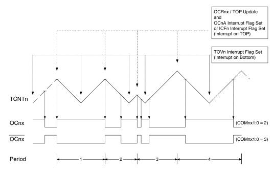
The Timer/Counter Overflow Flag (TOVn) is set each time the counter reaches BOT-TOM. When either OCRnA or ICRn is used for defining the TOP value, the OCnA or ICFn flag is set accordingly at the same timer clock cycle as the OCRnx Registers are updated with the double buffer value (at TOP). The interrupt flags can be used to generate an interrupt each time the counter reaches the TOP or BOTTOM value.
