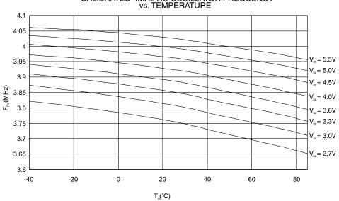
CALIBRATED 4MHz RC OSCILLATOR FREQUENCY vs. TEMPERATURE
