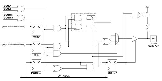
When the modulator is enabled the type of modulation (logical AND or OR) can be selected by the PORTB7 Register. Note that the DDRB7 controls the direction of the port independent of the COMnx1:0 bit setting.
