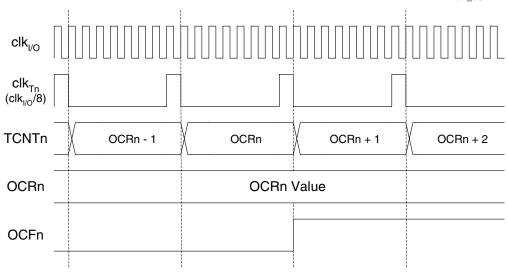
Figure 42. Timer/Counter Timing Diagram, Setting of OCF0, with Prescaler ( $f_{clk_l/O}/8$ )
