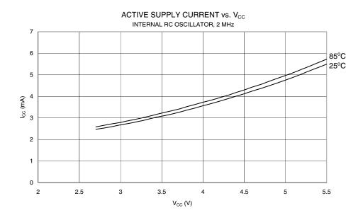
Figure 162. Active Supply Current vs. V<sub>CC</sub>, Internal RC Oscillator 2 MHz
