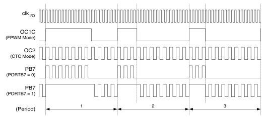
In this example, Timer/Counter2 provides the carrier, while the modulating signal is generated by the Output Compare unit C of the Timer/Counter1.
