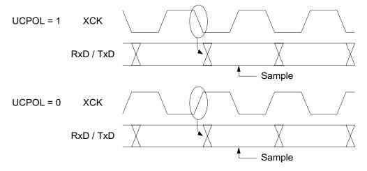
The UCPOL bit UCRSC selects which XCK clock edge is used for data sampling and which is used for data change. As Figure 80 shows, when UCPOL is zero the data will be changed at rising XCK edge and sampled at falling XCK edge. If UCPOL is set, the data will be changed at falling XCK edge and sampled at rising XCK edge.
