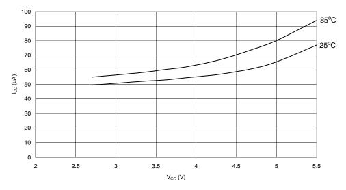
ANALOG COMPARATOR CURRENT vs.  $V_{\mbox{\scriptsize CC}}$
