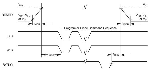
Figure 23. Temporary Sector Unprotect Timing Diagram
