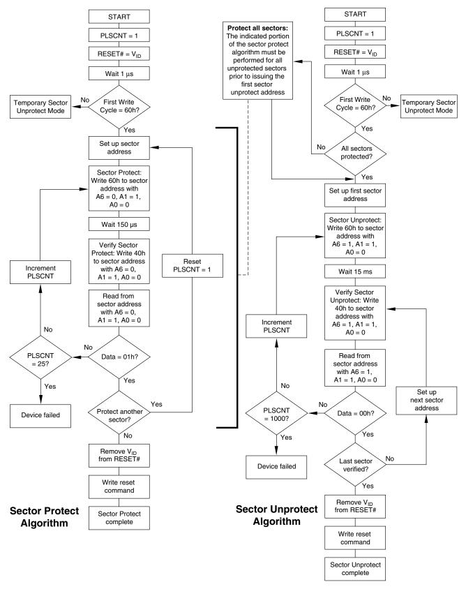
Figure 2. In-System Sector Protect/Unprotect Algorithms
