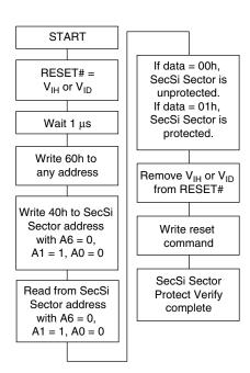
Figure 3. Secured Silicon Sector Protect Verify
