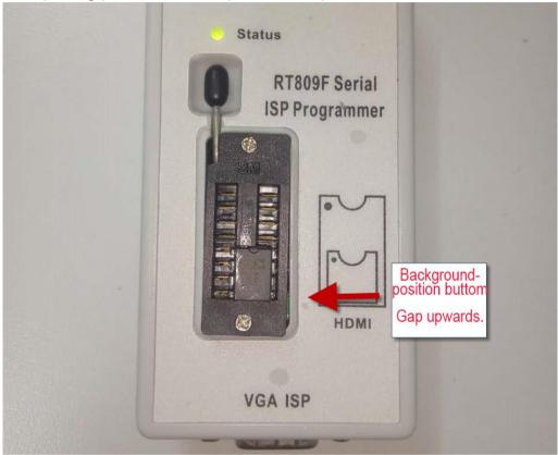
> The position of SOP encapsulation on the bounce board.
