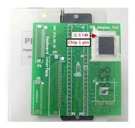
> The position of the chip on the socket;
