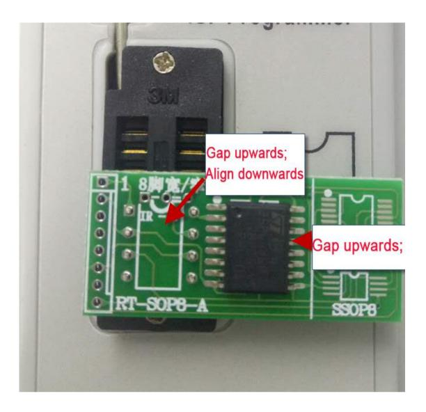
> If the power supply of the chip is 1.8V,it need to add the board.
