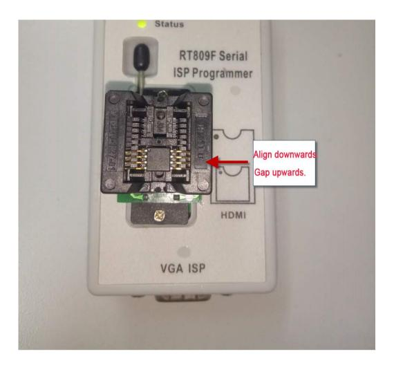
> The position of SOP encapsulation on the board.
