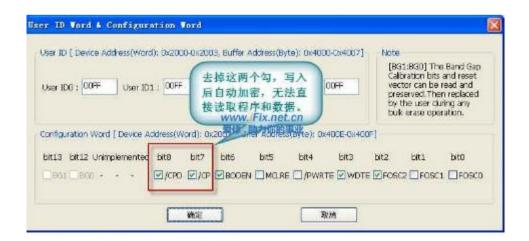
Note 2: If RT809F software hints that the program or data is encrypted after reading, then it is no need to save to be a file, not even write it into another chip.
