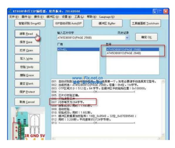
> Step 2: If the software hints "Flashing page is 256 bytes", then skip this step; if it hints "Flashing page is 264 bytes" then reselect the chip type and read again according to the following picture;
