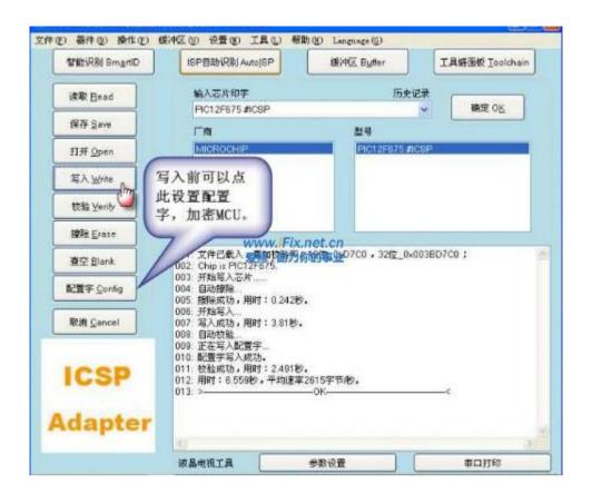
Note 1: The encryption is optional,MCU also can be used normally without being encrypted. If you cancel the /CP option of the configuration word before writing, the program area will encrypt automatically after finishing writing and verifying; if cancel the /CPD option the data area will encrypt automatically after finishing writing and verifying.
