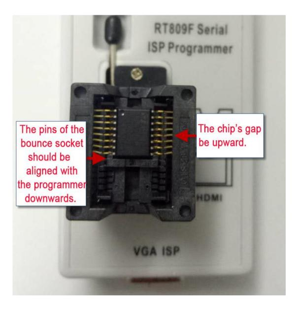
> The position of QSOP 16 pins encapsulation on the board.
