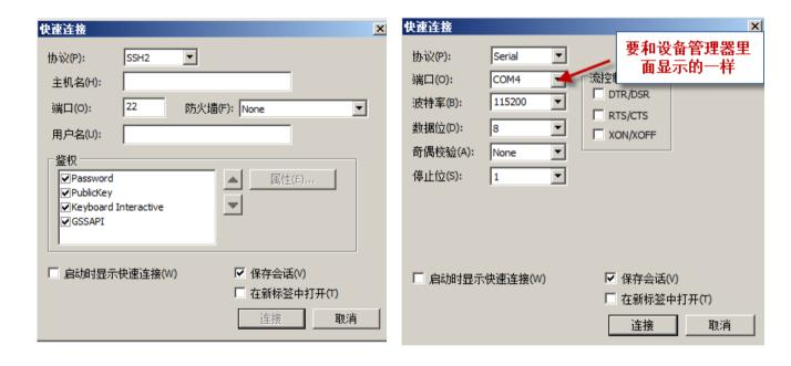
> Step 4 : Check the port in the device management;
