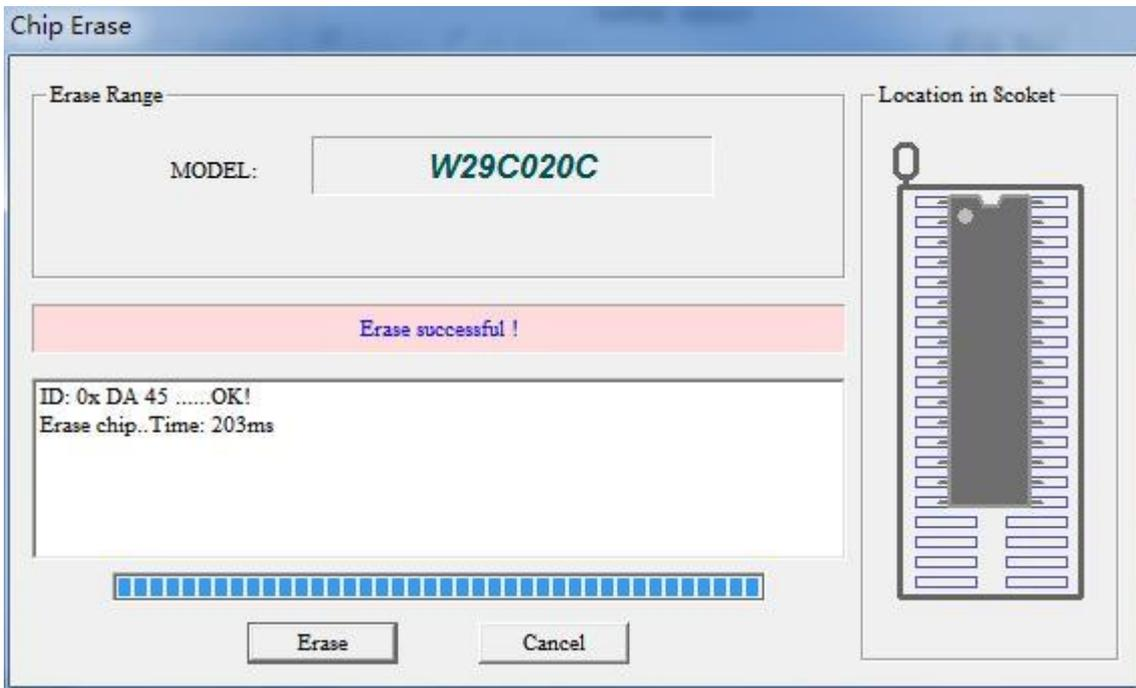
By default, the chip ID is checked before erasing. For a very few MCUs, some chips can not read the chip ID after being encrypted. In this case, cancel the ID check in the main interface, otherwise the ID check is incorrect. Click the [Erase] button in the dialog box, after erase is completed, the erase time is displayed.
