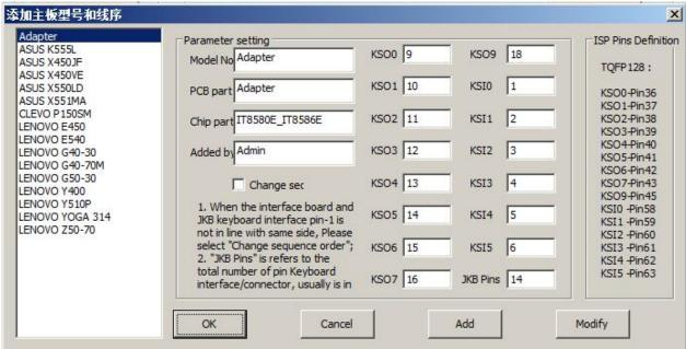
Laptop mainboard: Lenovo Y400,Board LA8691P,EC type IT8580. The other types like IT8586E, IT8586G, IT8585E,IT8587E and so on of TQFP128和BGA footprint EC,the reading and writing way:
