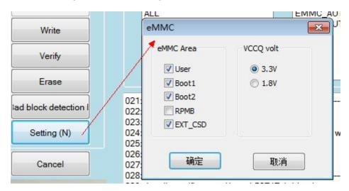
The left is the 5 partitions of EMMC, the "USER" is the user area, "RQMB" is the encryption area, the data in it can not come out so don't have to be chosen.
