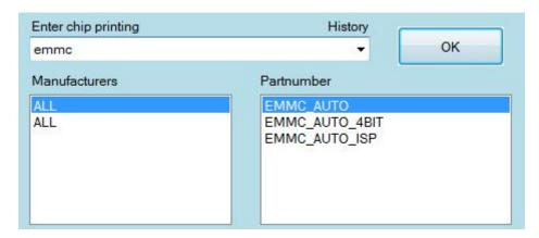
➤ EMMC\_AUTO\_4BIT:Slow-speed reading,but with high stability, higher successful rate,software default.
