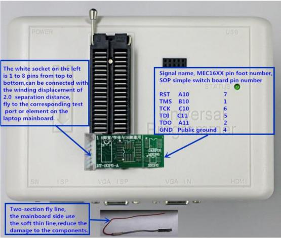
Connect the test point with the simple socket with the wire.
