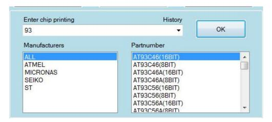
> Input "93" in the "Input Chip Printing Letter", select the detailed chip type at the lower right, then click "OK" after selecting.
