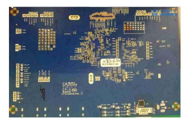
Step 1: In order to stop the main chip working (power supply,clock,restoration),the easiest way is crystal oscillator, ground the 2 pins of the crystal oscillator X0R2(beside the shielded wire extension cord) of the main chip;
