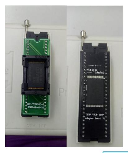
> Put the chip on the programmer, click the icon the type of the chip;
