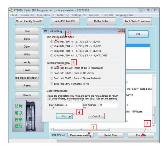
**Step 4**: After setting the parameter, click serial Print open the serial and electrify the mainboard in 2 seconds, the printing message will appear in the following dialog.
